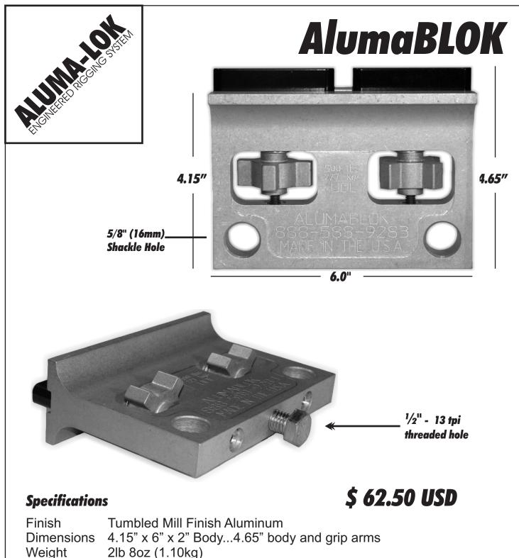
Load Rated **500 lb UDL (227 kg) Working Load Rating** (10:1 safety factor) Attachment (2) Shackle Hole 5/8" (16mm) & (1) ½"X 13TPI bolt hole
